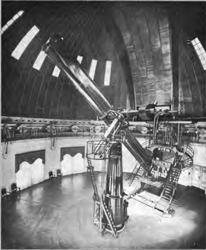
Great Double Telescope, Visual and Photographic, of the Potsdam Astrophysical Observatory. (See Sec. 51.)
